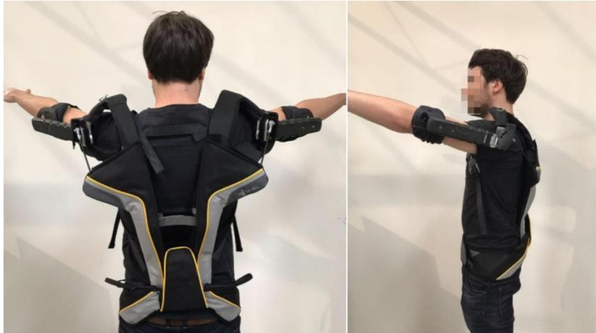
*Figure 1. SkelEx exoskeleton*
