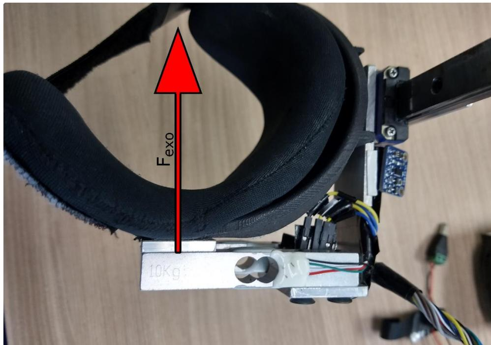
*Figure 2 Set up of the 1-axis force transducer. A single axis force transducer formed the connection between the arm cuff and the exoskeleton frame*
