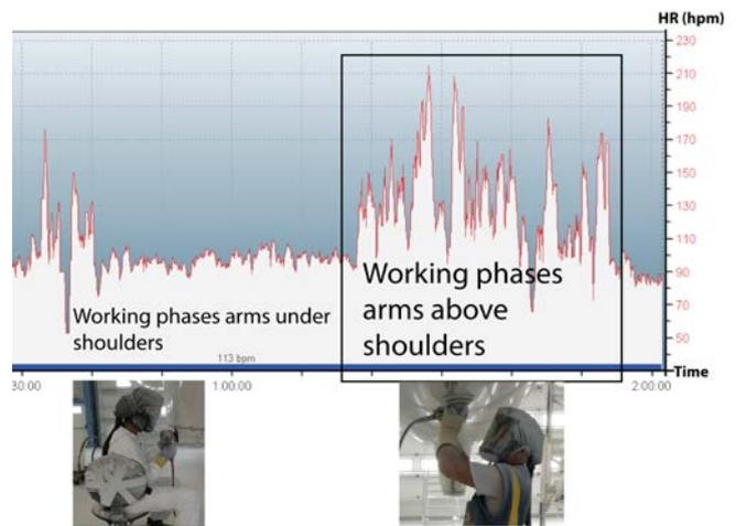
Fig. 1. (a) Evolution of heart rate for operator 1 during usual sanding process ; (b) Second measure after a break of 17 minutes. This curve will allow to identify extremum heart beats and average datas in the different levels of effort. The red curve indicates the evolution of heart rate, the coloured lines indicate intensity levels determined by the software.
