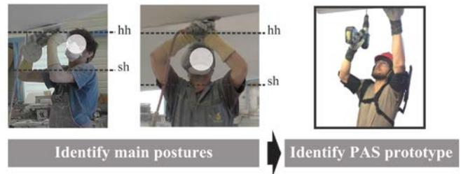
Fig. 5. Process of identifying an adapted PAD for the observed postures. Hh = Hands height; sh = shoulders height. The PAD selected is a prototype of Skel-Ex.
