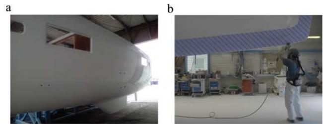
Fig. 1. (a) Side view of one catamaran hulls; (b) An operator is sanding the sealing edge. Hatches shows workzones for manual sanding.
