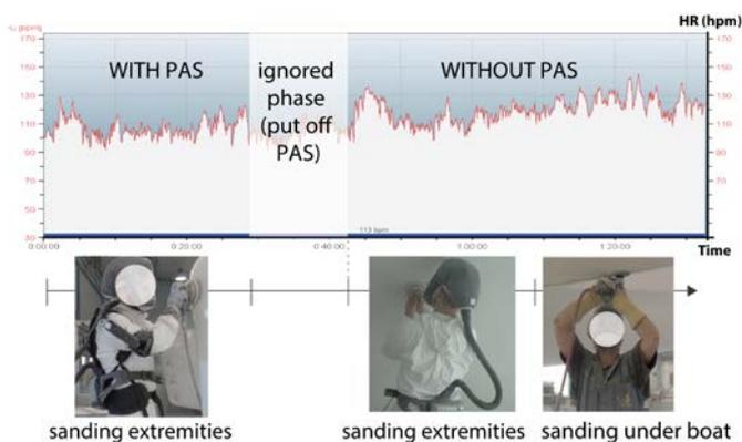
Fig. 6. Evolution of operator 8 heart rate measured for the usual tasks wearing the PAD at first then without PAD.
