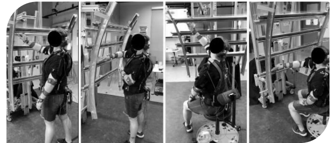
Fig 3a. Horizontal sealing tasks and starting postures (from left to right) a) standing sealing along upper stringer b) standing sealing along lower stringer c) seated sealing along upper stringer d) seating sealing along lower stringer
